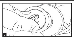
Reinsert the key into the cylinder. Hold assembly by the stems and work the key back and forth a few times to make sure everything is in proper order.
