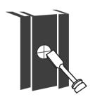
Drill a 1" (25mm) diameter hole in the door jamb.
