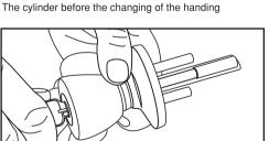
Push the cylinder all the way into the knob until you hear the spring retainers snap into place.
